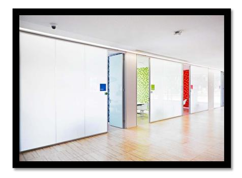
Privacy Smartglass, also referred to as privacy glass or switchable glass, is electric switchable glass with adjustable opacity. It uses electro-chromatic technology to interchange between transparency and an opaque state by applying voltage. Privacy Smartglass can change from clear to a frosted appearance at the flick of a switch while allowing light to pass through from both sides.
